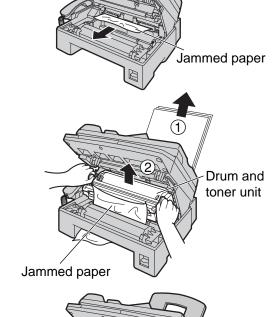
Remove the jammed paper from fuser unit by pulling it upwards carefully.
